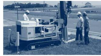
Geoprobe for soil and groundwater sampling
