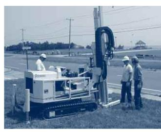
Geoprobe for soil and groundwater sampling
