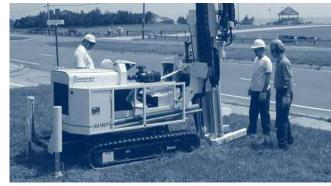
Geoprobe for soil and groundwater sampling
