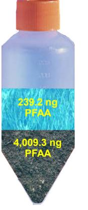
48-hour bottle tests: Soil Mass = 88.4 grams Groundwater Volume = 200 mL
