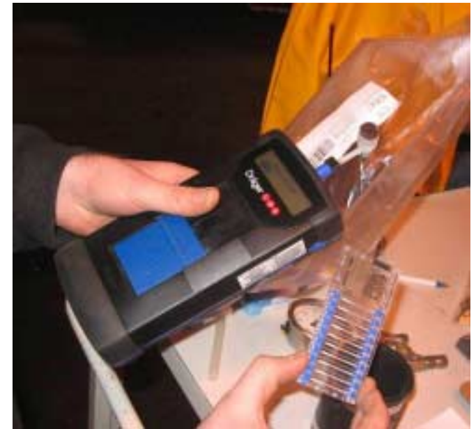
Optional compound specific analysis (Draeger chips)
